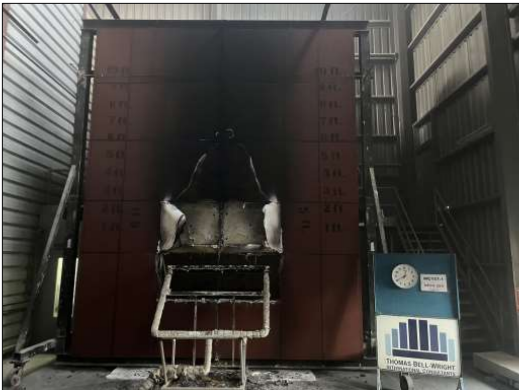
Picture 20: The specimen at the end of the observation period and end of the NFPA 285 test.
