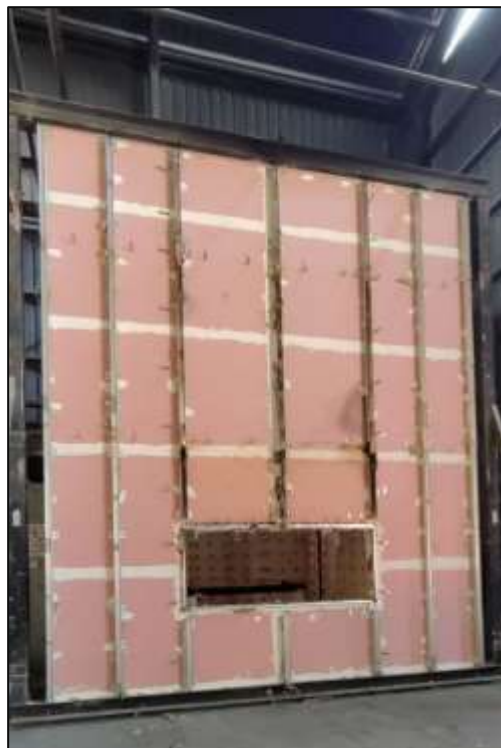
Picture 22: Assembly after the removal of panels and insulation system.
