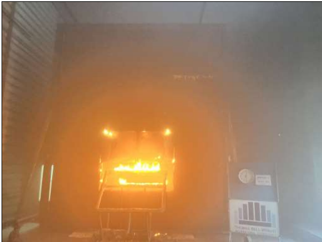
Picture 20: The specimen immediately after the gas was shut off, starting the observation period.
