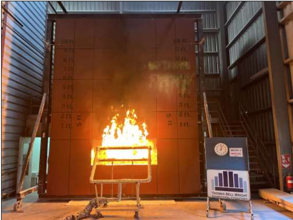
Picture 15: The specimen at 5:00 minutes and when the window burner was ignited.
